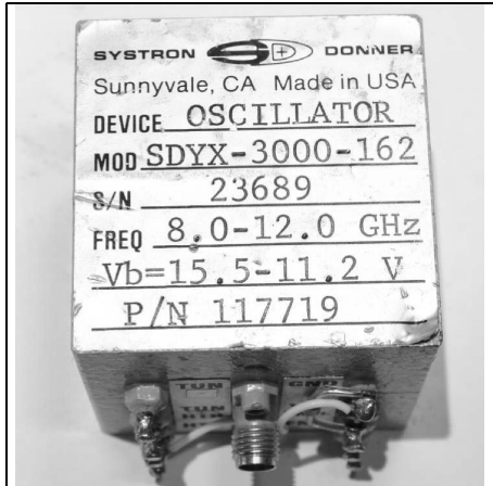
Fig 15: An example of a YIG oscillator requiring variable operating voltages.
